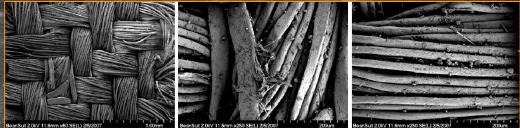
Electron micrographs showing damage to the outer layer of Alan Bean's Apollo 12 suit
